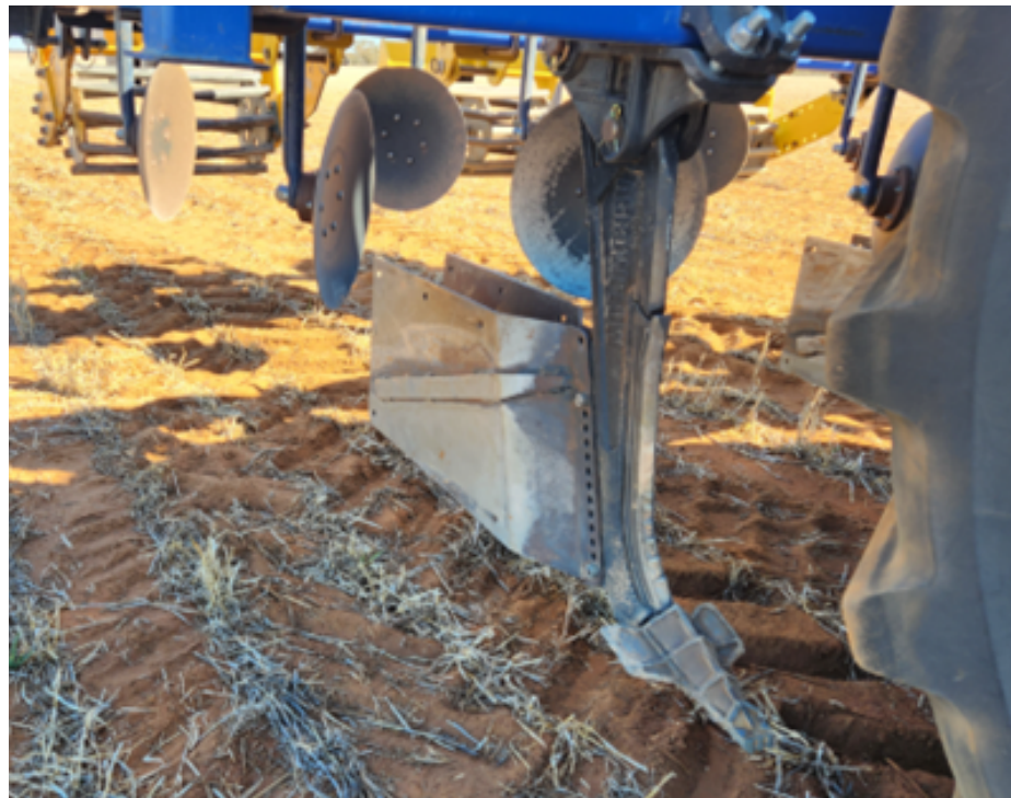
Inclusion plates attached to ripping tines allow top soil and organic matter to be transferred from the soil surface to deeper in the profile.
